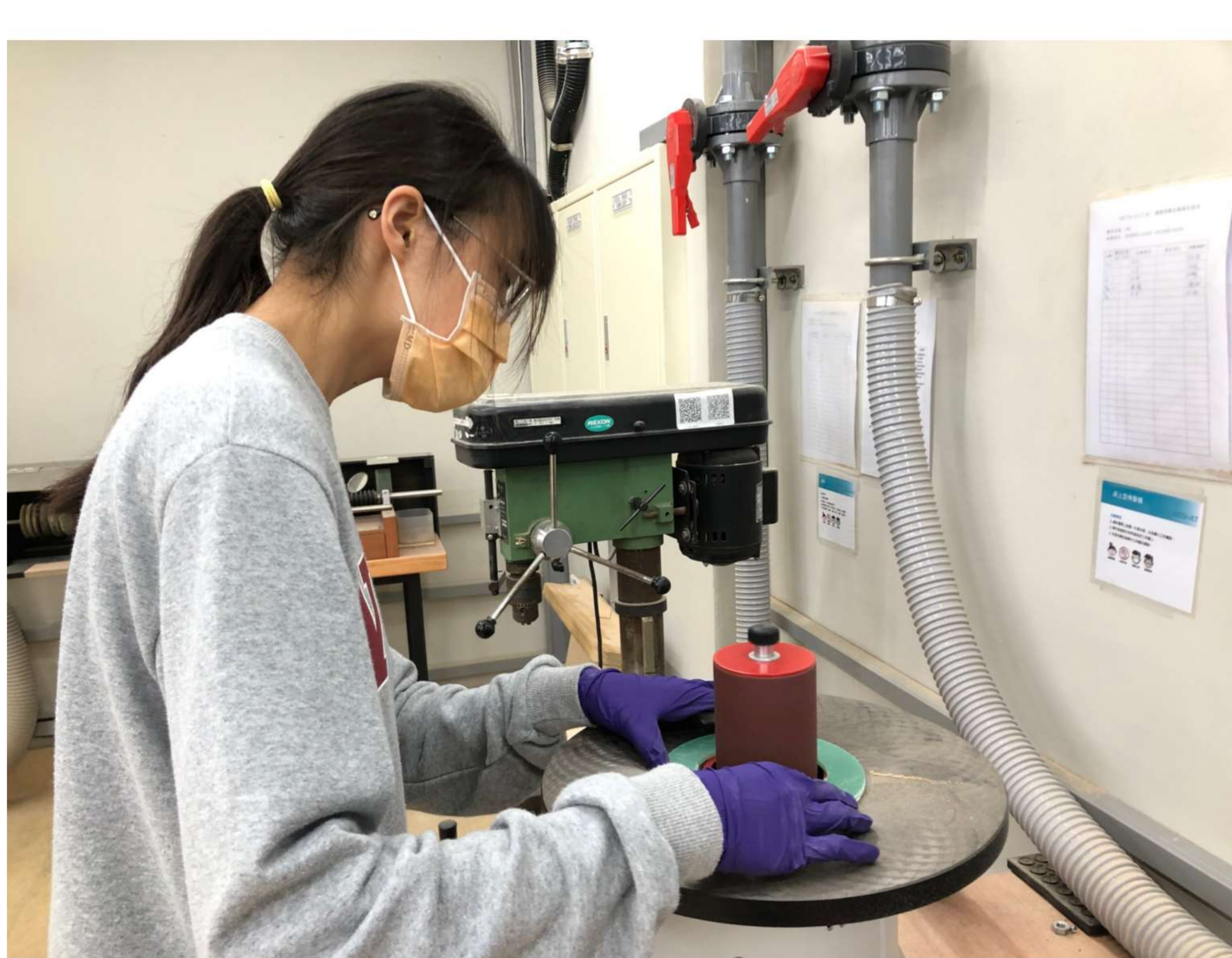
Use a sander to grind the size of the centering ring, so that it can match the diameter of the rocket airframe and the engine inner tube.
