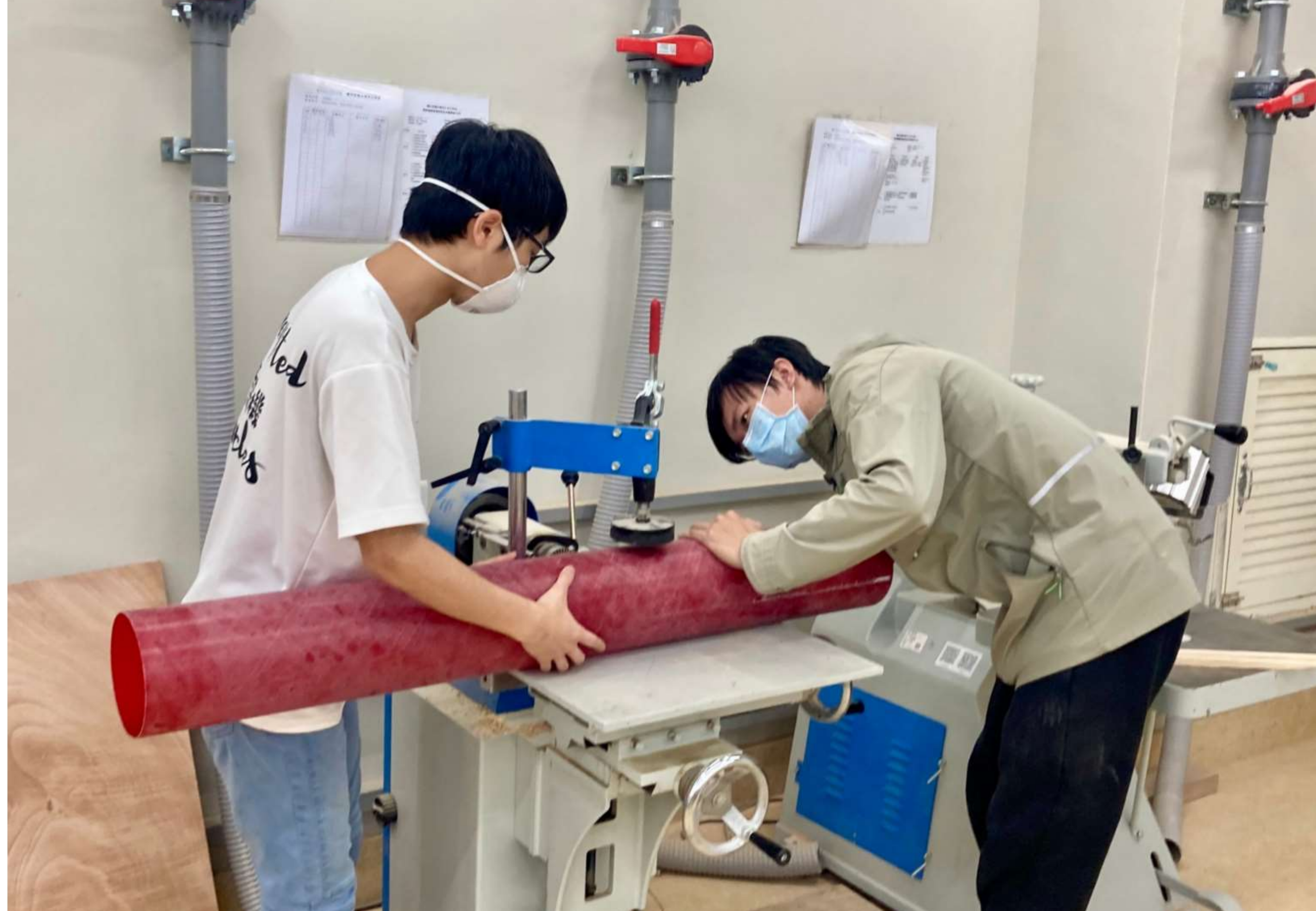
Manufacture The Joint Between The Rocket Airframe And Fins With A Horizontal Drill Press
